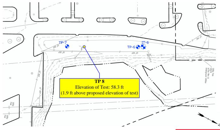
Notes: TP 8 tests were completed **ABOVE** the crushed gravel. Could not go any deeper as there was crushed gravel at 24-36in. Below the gravel was large stones/fragmented fill and could not auger the proper hole needed to complete the test at the proposed depth.
