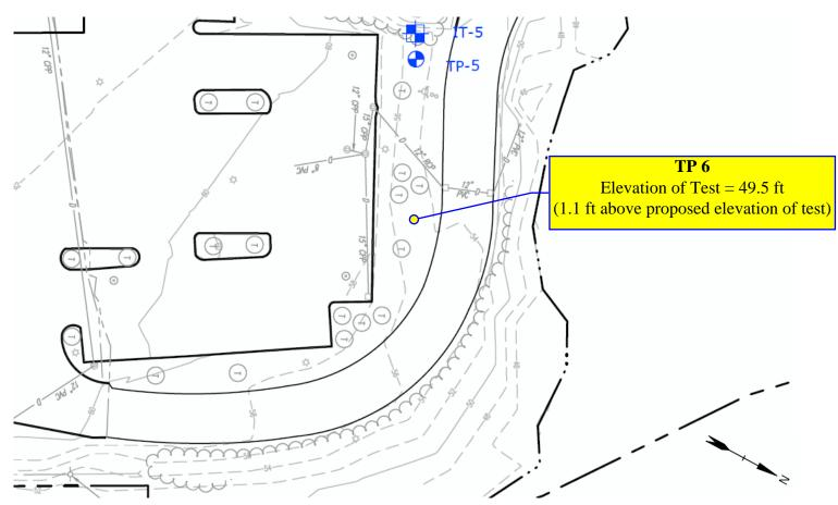
Notes: TP 6 tests were completed 1.1 ft above the proposed depth due to large stones/ fragmented fill and could not auger the proper hole needed to complete the test at the proposed depth.
